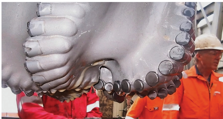
Fig. 1. The predominant method for well construction is drag bits equipped with PDC cutters.
