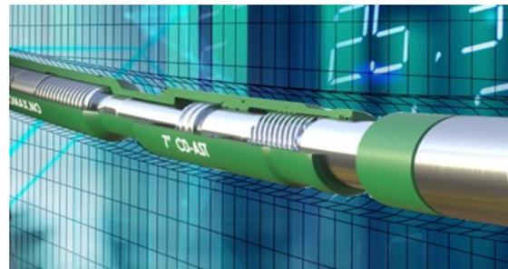
**Bottomhole Assembly (BHA):** The AST tool is typically placed in the BHA directly above the non-magnetic drill collars. If a roller-reamer or a stabilizer is placed near the AST, then it is recommended to position the AST below it. **DO NOT** position the AST in a string transition area e.g. between drill collars and heavy weight drill pipe (HWDP). Special recommendations are:
